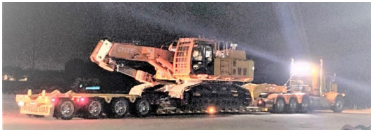
Fig. 20 Type II Test vehicle loaded with crane and counterweight, 68 Tons test
