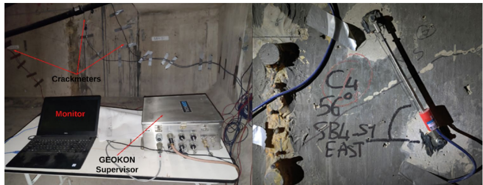
Fig. 15 Crackmeter sensors and system installation at Pier #4
