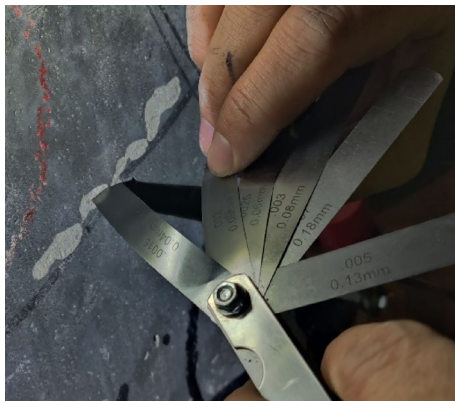
Fig. 33 Crack width initial reading measurement
