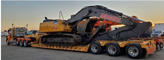
Fig. 19 Type II Test vehicle loaded with crane, 61 Tons test
