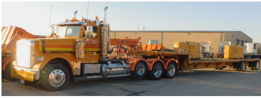
Fig. 18 Type I Test vehicle loaded with counterweights, 45 Tons test
